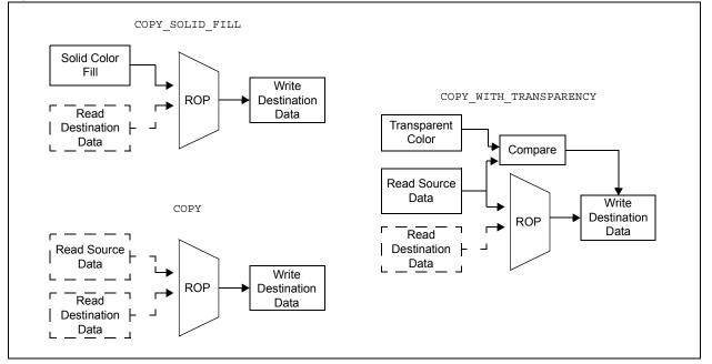
The source data is specified by Work Area 1 (W1ADR) and the destination by Work Area 2 (W2ADR). Depending on the type of copy operation, the source data and destination data are copied, modified or ignored.
