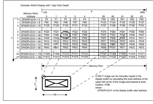
Figure 43-4 shows an example where a 64x24 display, with the display buffer starting at DPADR<23:0>, is initialized in memory. Memory pitch is calculated as: (64\*1)/8 = 8. If a 59x17 image is to be copied into the display buffer at location (2,6) or P386, the pixel address offset of P386 from the display buffer start address is calculated using Equation 43-2.
