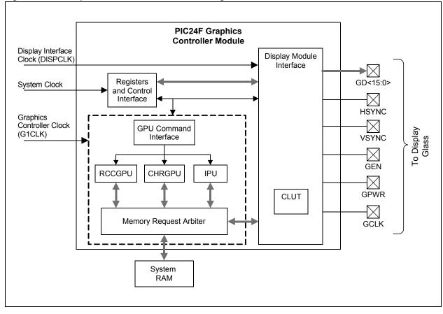
Figure 43-1: Graphics Module Pinout and Block Diagram
